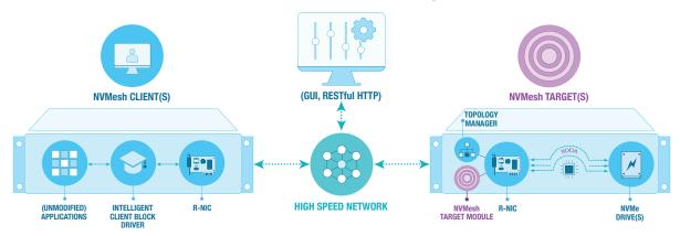
Thus, every compute node can have a local NVMe SSD (or multiple drives) and all the drives are pooled for use by the cluster. In the most simplistic form, with something like Lustre - 1/2 of each drive is used as a local burst buffer and 1/2 is reserved for the redundant copy of a peer. As a result, when a node fails, it's scratch is preserved and accessible by an alternate node - any node on the fabric.
