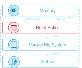
Once the burst (checkpoint) is complete, the written data is "drained" to the larger, slower pool of storage making up the majority of the file system. This allows checkpoints to finish rapidly so that systems meet SLAs and the time between checkpoints is used to move the stored checkpoints to longer-term storage pools.
