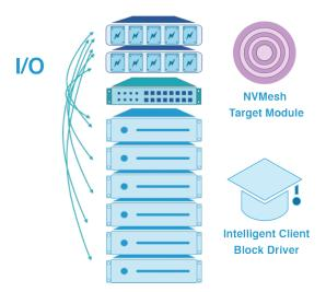
In a disaggregated model, specific "target" storage nodes supply storage to the "client" compute nodes. Target nodes can be based on JBOFs (Just a Bunch of Flash) or on dedicated servers with a large (usually at least 24) number of drives. To provide access to this many drives, target nodes usually have RNICs with up to eight 100Gb/s ports. Client nodes will have local storage only for the operating system and use RNICs of up to two 25Gb/s ports.
