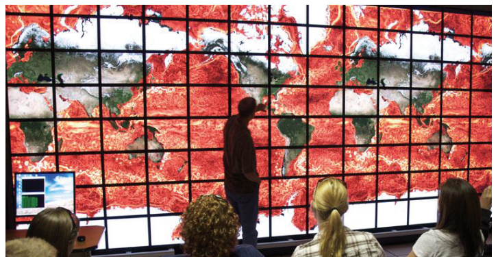
The hyperwall allows researchers to view and interact with tremendously large simulations at a resolution normal computer screens are simply not capable of.
