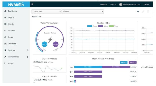
The ability to observe the underlying volume provides clear demonstration that the data written to the ELECT volume 'mtv' is being written to the Write Cache volume 'wcv' first and then is being read from it to be destaged to the QLC EC volume 'qlc'. The metadata access is very small compared to the data operations.
